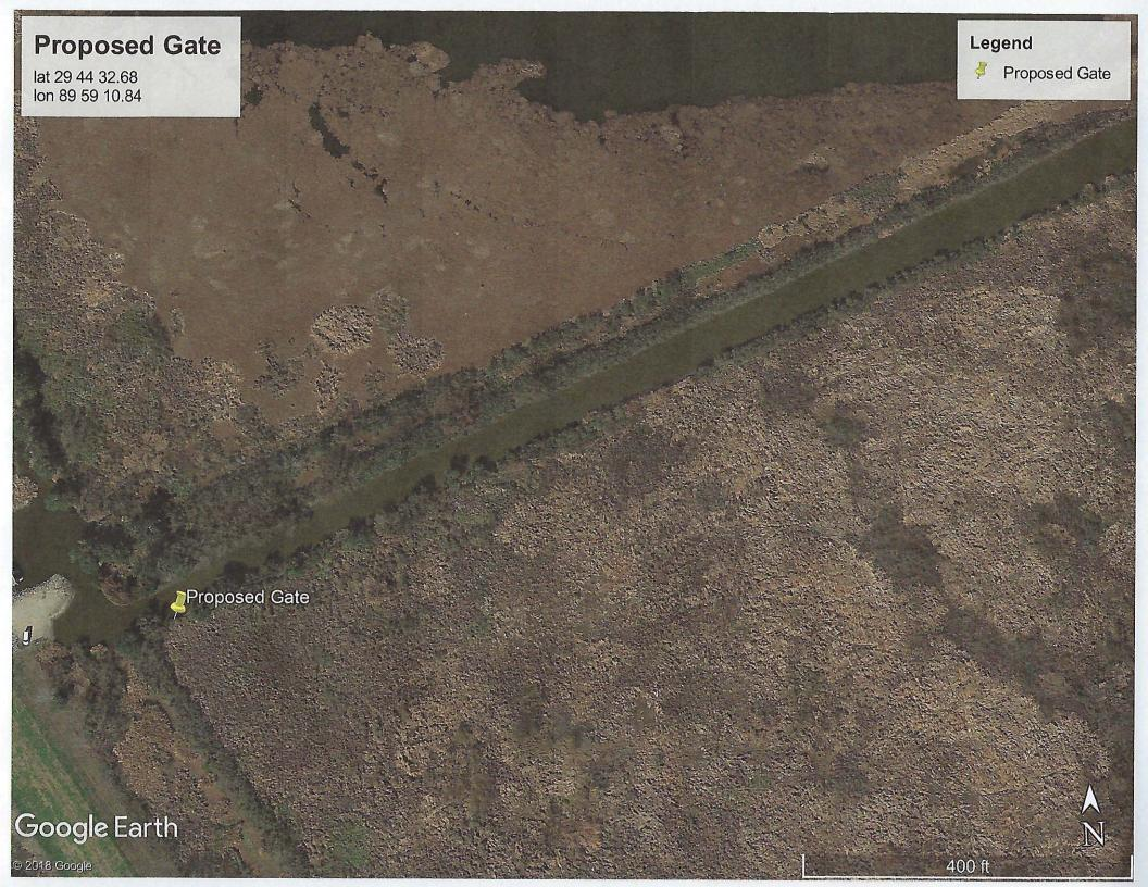
IAN VIEW Average Depth of CANVAL 3.2 Feet GAte will Average High Tipe RANGE Be completely 15 + 1.2 Feet OUT of The water AND Average Low Time Range VISIBLE At All 15 -0.03 Feet TO .049 Times Feet
